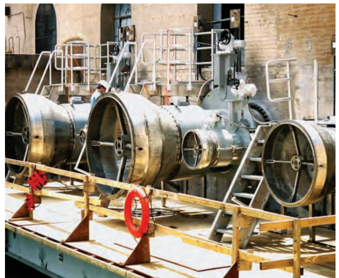
Eleven Mile Dam, Colorado, USA—Five Ring Jet Valves (8", 16", 30", and two 48") and Five Rotovalve® Cone Valves (8", 16", 30", and two 48").
