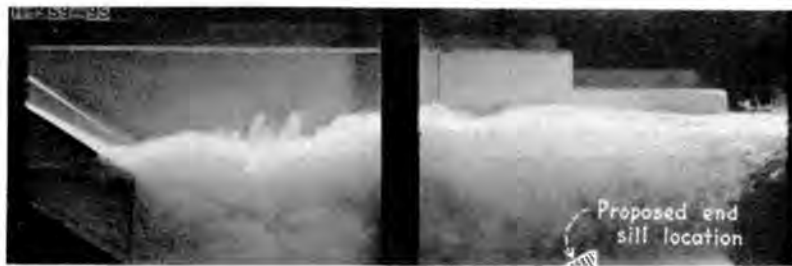
(c) Stilling action with recommended converging walls
