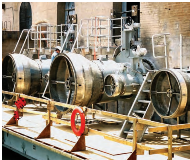
Eleven Mile Dam, Colorado, USA—Five Ring Jet Valves (8", 16", 30", and two 48") and Five Rotovalve® Cone Valves (8", 16", 30", and two 48").
