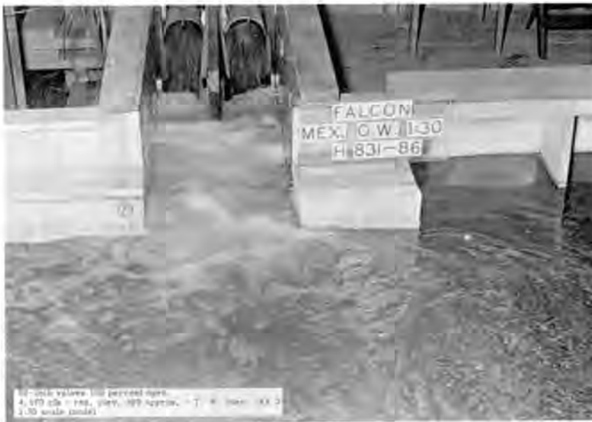
FIG. 23.—MEXICAN OUTLET WORKS - FALCON DAM
